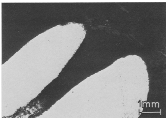
Fig. 2. Coherent gadolinium dendrites deposited at 870 °C after stabilization of the 75 LiF-25 mol% GdF_3 electrolyte by oxyfluorocomplexes
